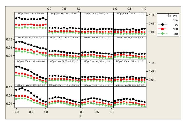
**Figure 14.** Plot of the standard errors of the estimators of the indices  $MC'_{pk}$ ,  $MC'_{pmr}$  and  $MC'_{pmk}$  for three sample sizes, various common values  $\mu$  for  $\mu_1$  and  $\mu_2$ , and various values of  $\sigma_1^2$  and  $\sigma_2^2$  with  $\sigma_{1,2} = 0.4$
