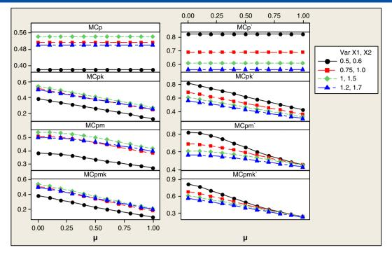
Figure 7. Plot of the indices  $MC_{pr}$ ,  $MC_{pkr}$ ,  $MC_{pmr}$ ,  $MC'_{pr}$ ,  $MC'_{pr}$ ,  $MC'_{pmr}$ , and  $MC'_{pmr}$  for various common values  $\mu$  for  $\mu_1$  and  $\mu_2$  and various values of  $\sigma_1^2$  and  $\sigma_2^2$  with  $\sigma_{1,2} = 0.2$
