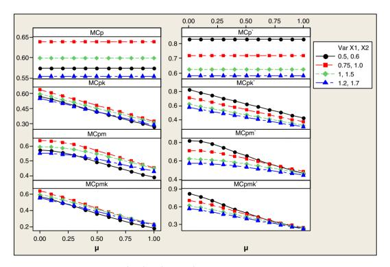
Figure 6. Plot of the indices MC<sub>p</sub>, MC<sub>pk</sub>, MC<sub>pm</sub>, MC<sub>pm</sub>, MC<sub>pk</sub>, MC<sub>pm</sub>, MC<sub>pm</sub>, MC<sub>pm</sub>, and MC<sub>pm</sub>, for various common values  $\mu$  for  $\mu_1$  and  $\mu_2$  and various values of  $\sigma_1^2$  and  $\sigma_2^2$  with  $\sigma_{1,2} = 0.1$
