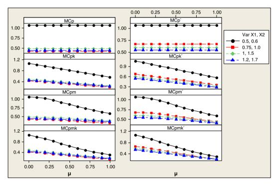
Figure 8. Plot of the indices  $MC_{pr}$ ,  $MC_{pkr}$ ,  $MC_{pmr}$ ,  $MC'_{pkr}$ ,  $MC'_{pkr}$ ,  $MC'_{pmr}$  and  $MC'_{pmr}$  for various common values  $\mu$  for  $\mu_1$  and  $\mu_2$  and various values of  $\sigma_1^2$  and  $\sigma_2^2$  with  $\sigma_{1,2} = 0.3$
