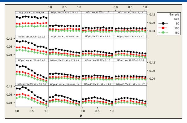
**Figure 13.** Plot of the standard errors of the estimators of the indices  $MC'_{pk}$ ,  $MC'_{pmr}$  and  $MC'_{pmk}$  for three sample sizes, various common values  $\mu$  for  $\mu_1$  and  $\mu_2$ , and various values of  $\sigma_1^2$  and  $\sigma_2^2$  with  $\sigma_{1,2} = 0.3$
