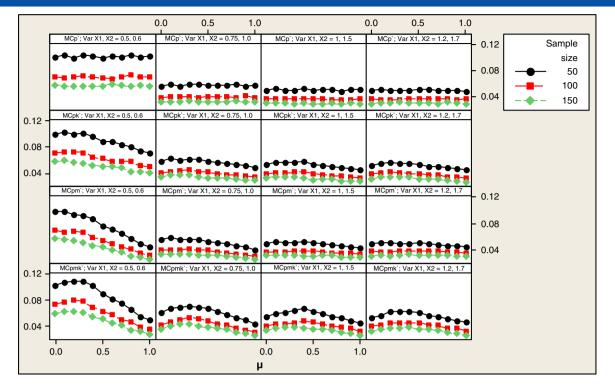
**Figure 15.** Plot of the standard errors of the estimators of the indices  $MC'_{pk}$ ,  $MC'_{pmr}$  and  $MC'_{pmk}$  for three sample sizes, various common values  $\mu$  for  $\mu_1$  and  $\mu_2$ , and various values of  $\sigma_1^2$  and  $\sigma_2^2$  with  $\sigma_{1,2} = 0.5$
