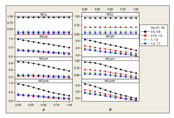
**Figure 10.** Plot of the indices  $MC_{pk}$ ,  $MC_{pm}$ ,  $MC_{pmk}$ ,  $MC'_{pm}$ ,  $MC'_{pm}$ , and  $MC'_{pmk}$  for various common values  $\mu$  for  $\mu_1$  and  $\mu_2$  and various values of  $\sigma_1^2$  and  $\sigma_2^2$  with  $\sigma_{1,2} = 0.5$
