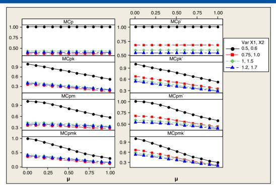
**Figure 9.** Plot of the indices  $MC_{pr}$ ,  $MC_{prk}$ ,  $MC_{prm}$ ,  $MC'_{prk}$ ,  $MC'_{prm}$ , and  $MC'_{prm}$  for various common values  $\mu$  for  $\mu_1$  and  $\mu_2$  and various values of  $\sigma_1^2$  and  $\sigma_2^2$  with  $\sigma_{1,2} = 0.4$
